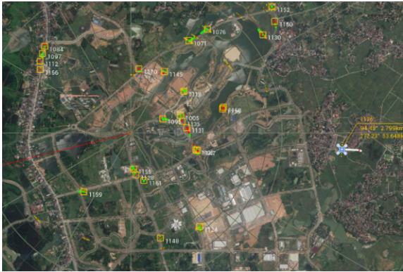
Figure 19. “Discrete clutter” and “Drone” on radar screen (recognize a drone from 3km)
