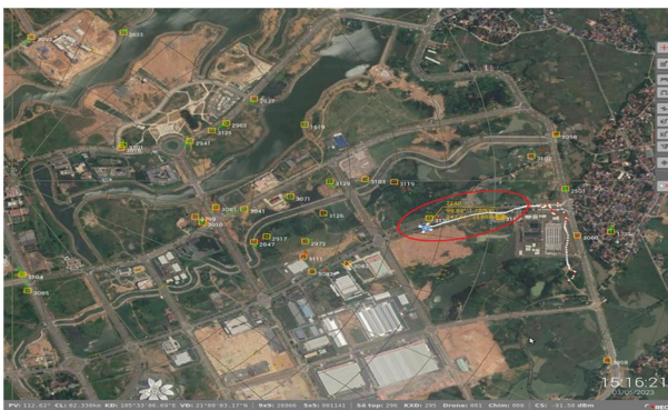
FIGURE 16 Classification of a drone moving along the street (in the red ellipse) from a range of 1.7 km using the Doppler diversion feature.
