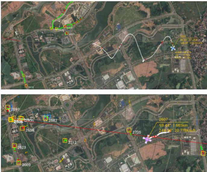
Figure 20. Test results with different moving scenarios: drone moves in a sinusoidal trajectory (above) and along the street (below)
