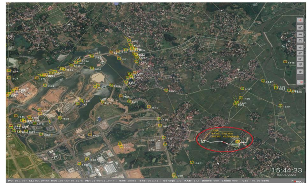
FIGURE 8 Detection of the DJI Phantom 4 by the radar (in the red ellipse).
