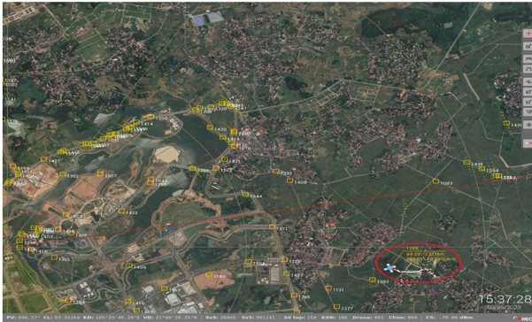
FIGURE 14 ‘Discrete clutter’ and ‘Drone’ on the radar screen. Classification of a drone (in the red ellipse) from 3.5 km by using the ‘Street Model’.
