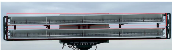
FIGURE 6 The manufactured antenna with flares (in the red rectangles).
