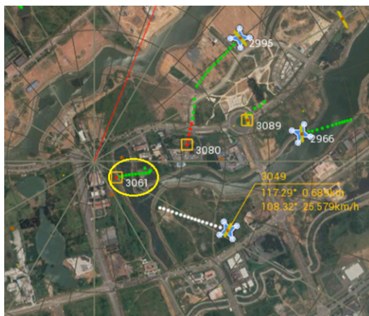
Figure 21. Three drones (inspire 2, phantom 4 and mavic 3) and a bird (inside the circle) in a test
